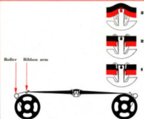
with the finger. Before doing so, move the ribbon arm as far as it will go away from the spool towards the centre of the machine.
